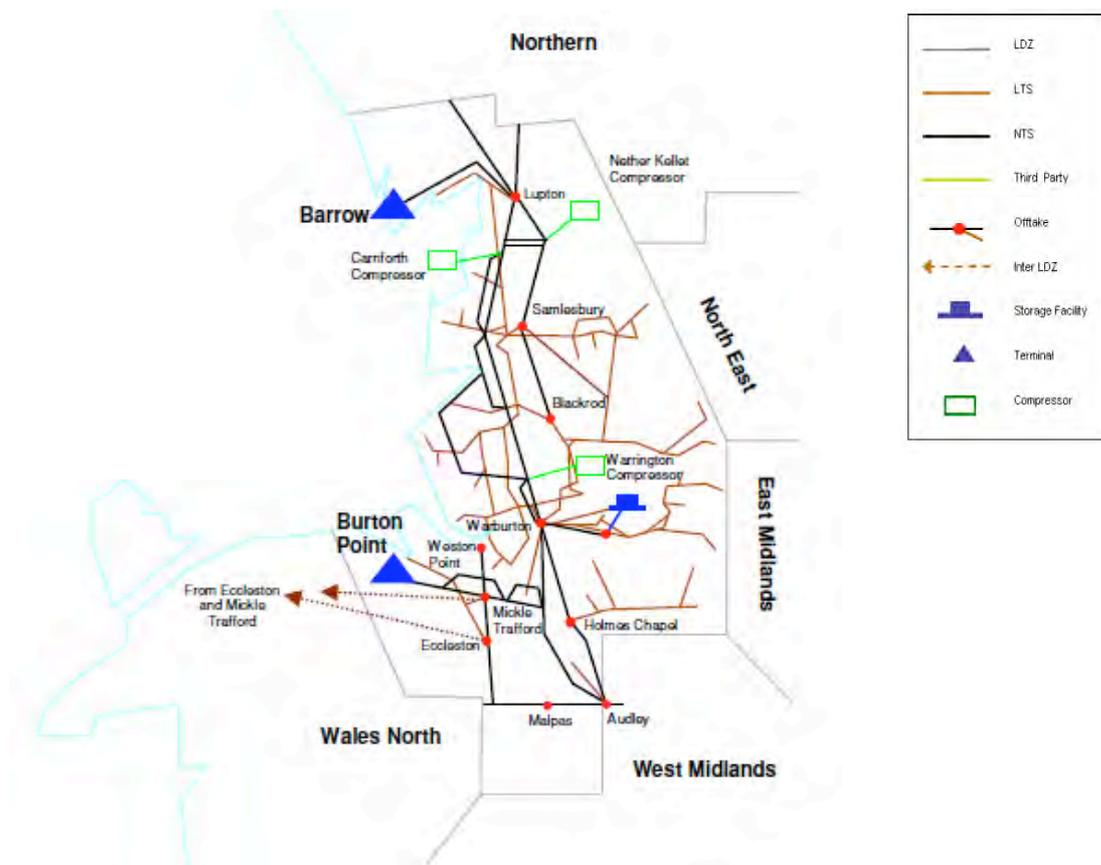
The NTS transports gas, at pressures up to 85 bar, from terminals at Barrow and Burton Point to NTS off takes. At the NTS off takes, gas travels into the High Pressure distribution system (HP), shown as LTS above. This tier transports gas to the lower pressure tiers and has gas
